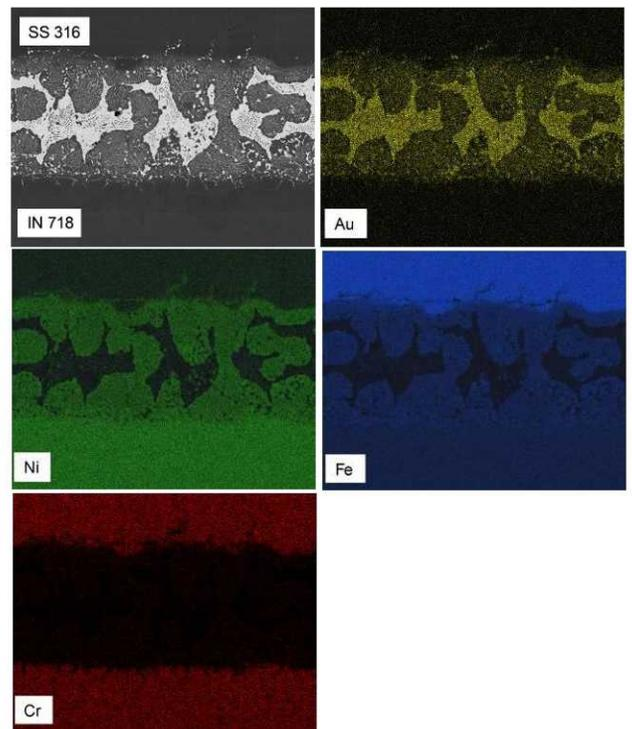
**Figure 8.** FESEM BSE image of Nioro brazed SS316L to IN718 after long term exposure at 900 K for 1000 hours with energy dispersive spectroscopy elemental maps for Au, Ni, Fe, and Cr.
