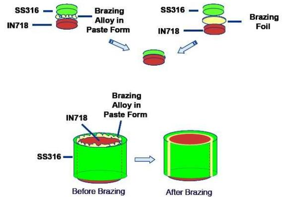
**FIGURE 2.** Illustration of various Brazing Approaches using Paste and Foil to Evaluate the Process and the Compatibility of various Commercial Braze Alloys with SS316L and IN718 alloys.
