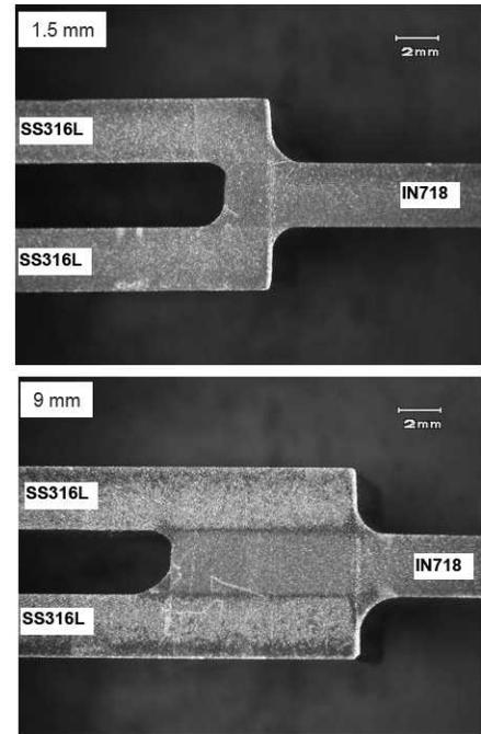
**Figure 11.** Cross Sections of SS316L/IN718 Double-lap Shear Specimens Brazed with Niore with (a) 1.5 and (b) 9 mm Overlaps.
