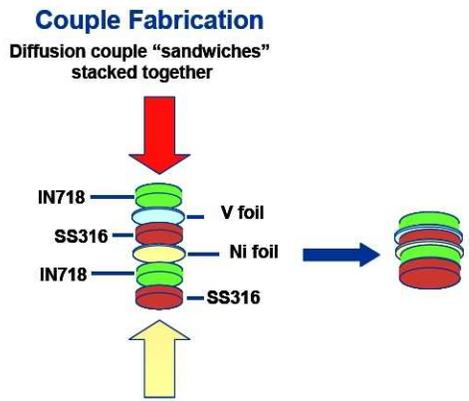
**FIGURE 1.** Illustration of Hot Pressing Sequence to Produce Multiple, Dissimilar Metal Diffusion Couples.
