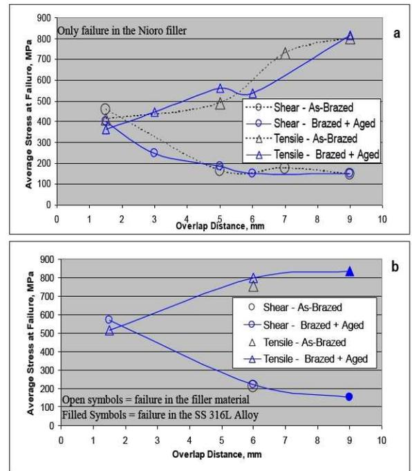
**Figure 12.** Average Shear Stress and Tensile Stress as a Function of Overlap Distance with (a) Niore: Failure Occurred only in the Brazing Filler Metal, and (b) Palniro-7: Failure Transition from Filler to SS316L Base Metal at the 9 mm Overlap.
