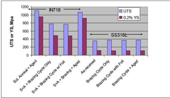
**FIGURE 10.** Effect of the Brazing, Anneal, Age Thermal Cycles, and Contact with Braze Material on the Mechanical Properties of IN718 and SS316L at 830K.
