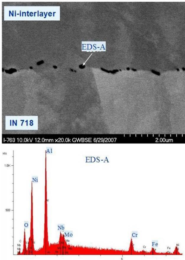
**Figure 5.** FESEM Image and Energy Dispersive Spectrum Confirming the Presence of  $\text{Al}_2\text{O}_3$  Particles Trapped in the Fine Pores Formed at the IN718/Ni-Interlayer Interface after Hot Pressing at 1150 K for 2 Hours at 90 MPa.
