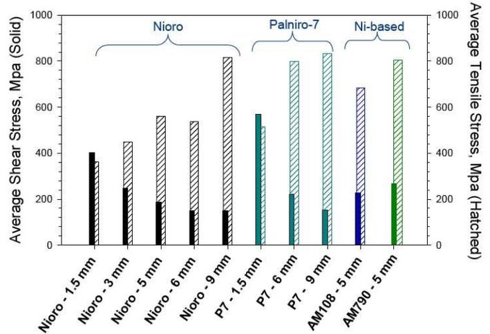
**Figure 14.** Average Shear and Tensile Stress at Failure as a Function of Braze Materials and Overlap Distances. All Brazed Specimens Were Aged before Testing.
