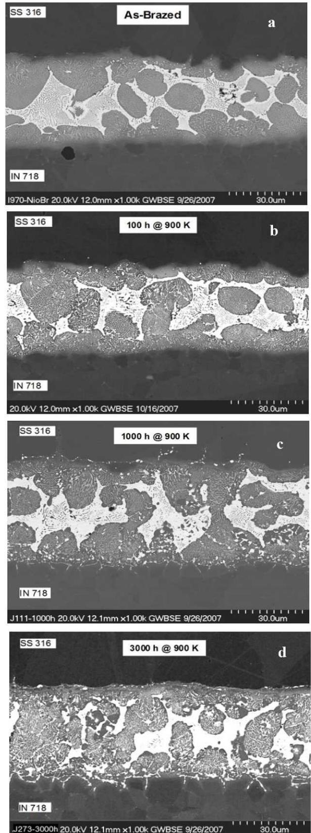
**Figure 6.** FESEM BSE Images of Niobium Brazed SS316L to IN718 in the (a) as-Brazed Condition, and after Long Term Exposures at 900 K after (b) 100, (c) 1000 h, (d) 3000 Hours.
