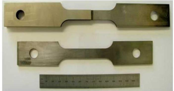
**FIGURE 3.** Typical Brazed Double-Lap Shear and Control Specimens Used for Testing at 830K.
