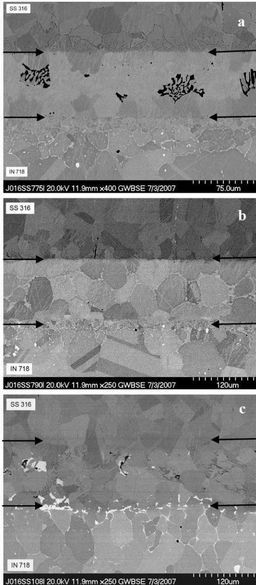
**Figure 9.** FESEM Images Showing Approximate Location of the Original Interfaces, Features of the Brazing Bonds and Reaction near the Bond Interfaces after the Brazing Process using (a) AM775, (b) AM790, and (c) AM108 Brazes.
