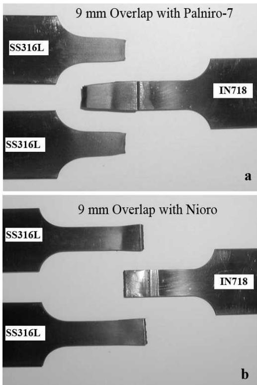
**Figure 13.** Different Types of Failures with same 9 mm Overlap (a) Failure in the Base Metal with Palniro-7 (SS316L), and (b) Failure in the Nioro Brazing Filler Metal.
