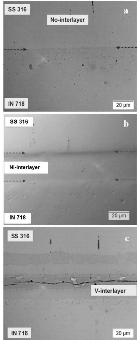
**Figure 4.** Optical Micrographs of Hot Pressed at 1150 K for 2 hours at 90 MPa Couples: (a) SS316L to IN718, (b) SS316 to Ni-interlayer to IN316, and (c) SS316L to V-interlayer to IN718. Bond Interface Indicated with Arrows.
