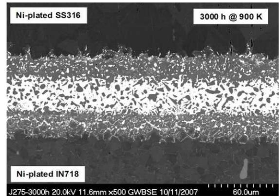
**Figure 7.** FESEM BSE Image of Ni-plated SS316L and IN718 plates brazed with Nioro after a 3000 Hours Exposure at 900 K.
